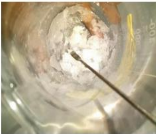
Figure 5. Shape of zinc sulfate after filtration and evaporation.
