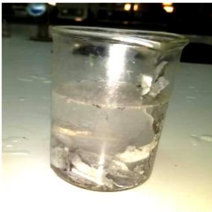
Figure 4. Immersed zinc shell of batteries in sulfuric acid.
