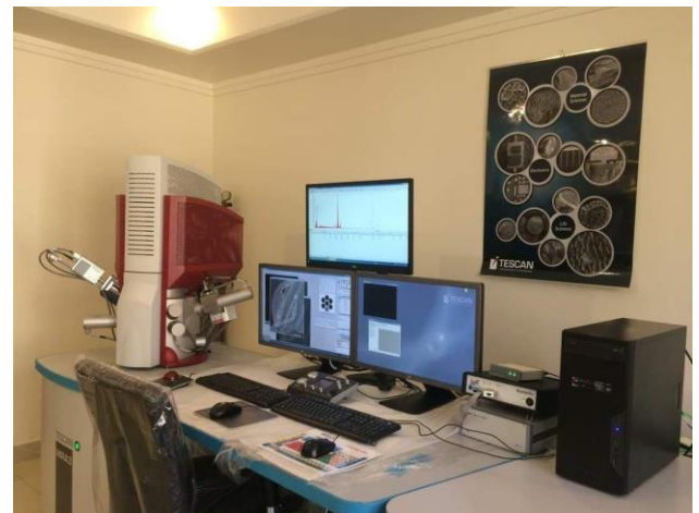
Figure 2. SEM with EDS systems.
