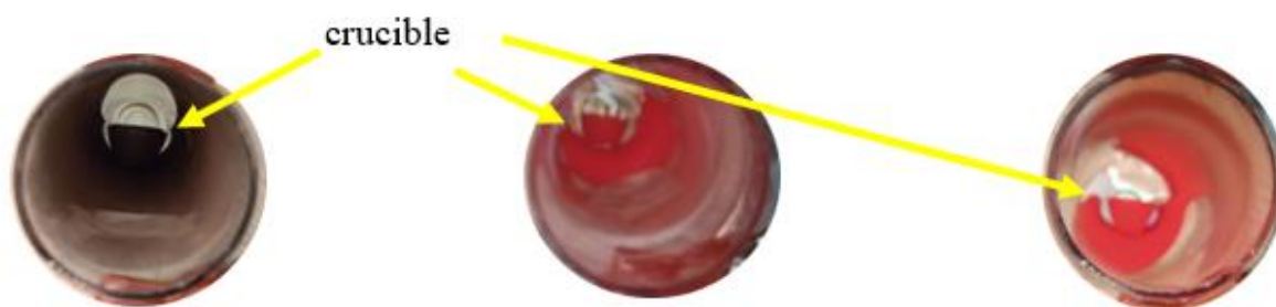
Figure 2: The PPW samples coal under a 600 °C tube furnace.
