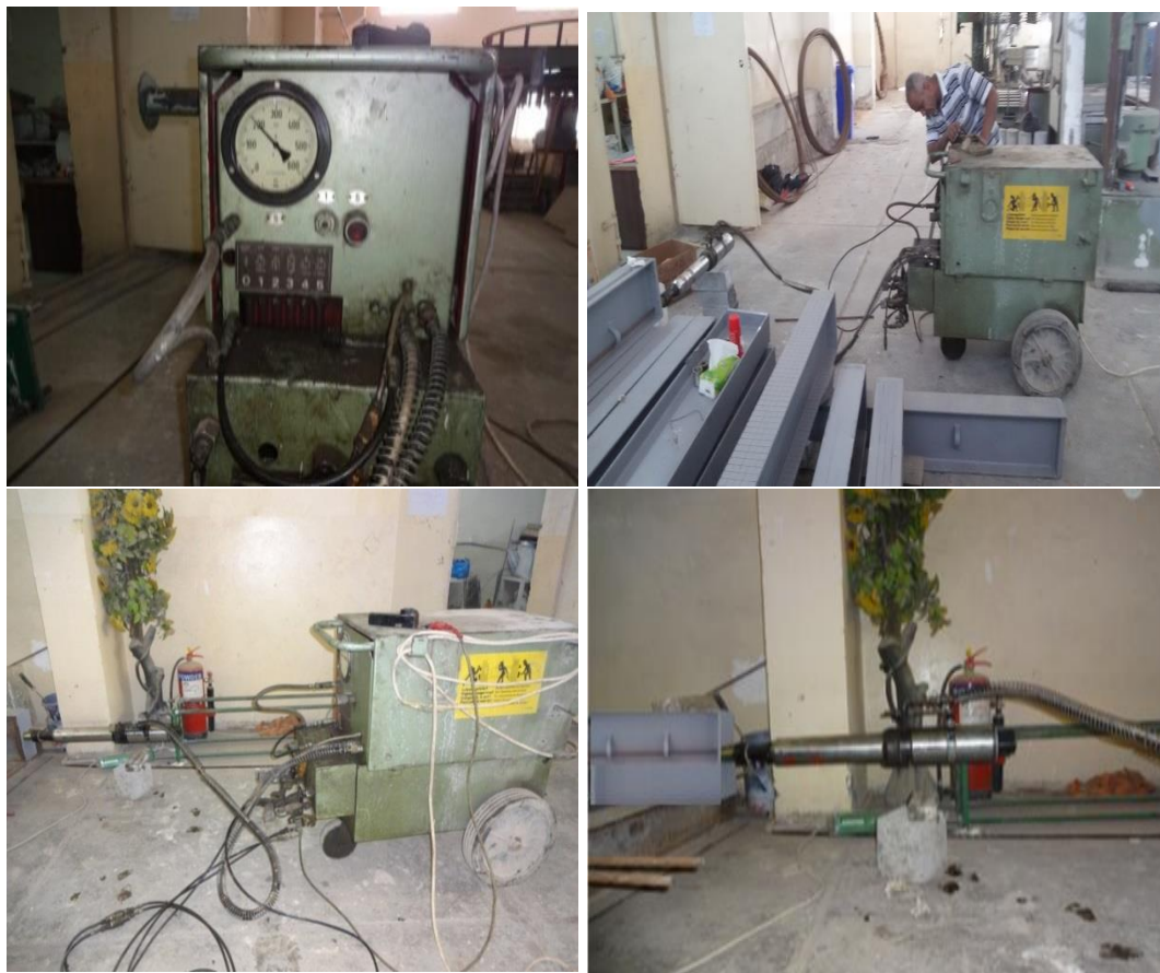
Figure (6) Hydraulic machine and single strand jack prestressing strand.
