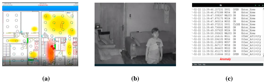
Fig. 10. Screenshots of Safe Smart Home Scenario 1. (a) The computer screen displays each sensor event. (b) The window's status bar at the bottom shows that residents typically move around the home during the hours that are recognized as such. (c) The sensor event visualizer in real-time displays the home's sensor status during the scenario. The kitchen (bottom right corner of the home) is where the occupant is seen.
