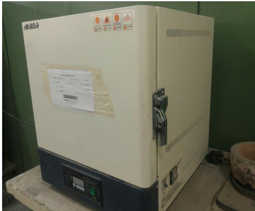
Figure 5. Special oven used for burning soil samples at high temperature, used in this study In Diyala University-collage of Engineering-Civil Engineering Department laboratories
