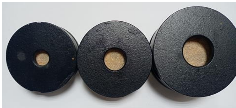
Figure 3: Explain the samples prepared to test with the coating silicon sand ( \text{SiO}_2 ).
