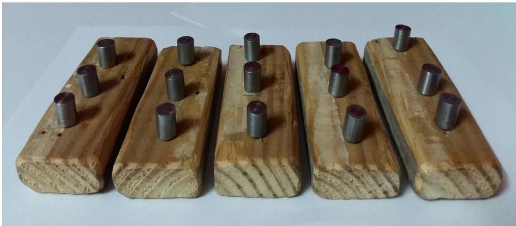
Figure 3. Hold the steel samples on the wood before shot peening
