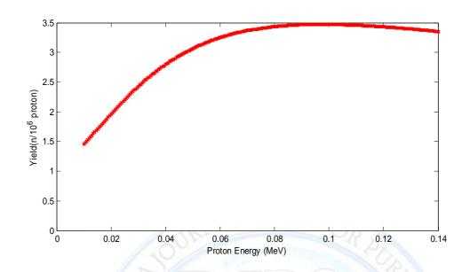
Fig.(4): Neutron Yield for <sup>50</sup>Cr(p,n)<sup>50</sup>Mn reaction
