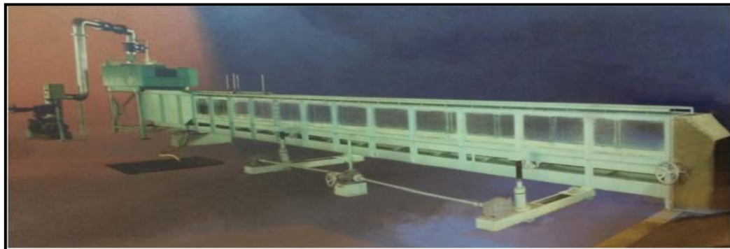
Figure 1 The flume that was employed in this investigation.
