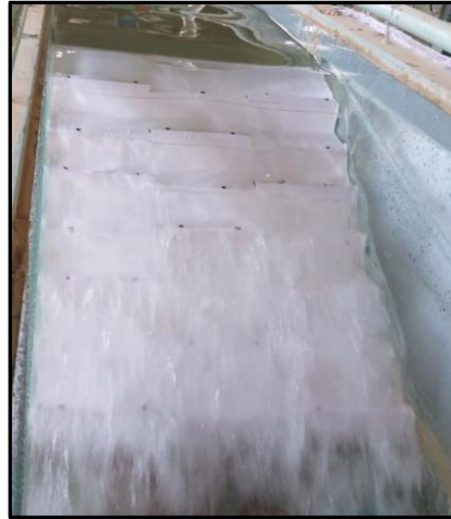
Figure 4 Transition flow regime Zig-Zag Pooled Step, N_s= 7 , Q = 12 L/s.
