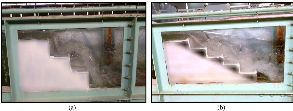
Figure 3 Nappe flow regime; (a) Nappe Flow, Fully Pooled Step, N_s= 5 , Q = 7 L/s and (b) Nappe Flow, Fully Pooled Step, N_s= 3 , Q = 12 L/s
