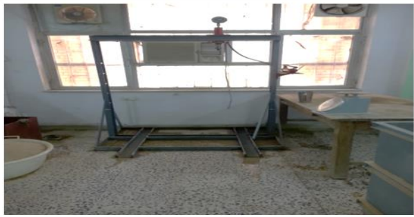
(a): Steel frame and hydraulic jack
