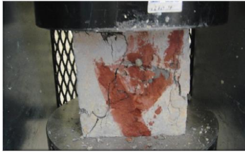
Figure 14. The shape of failure after loading for a cube with GL51 and fired for 3hr
