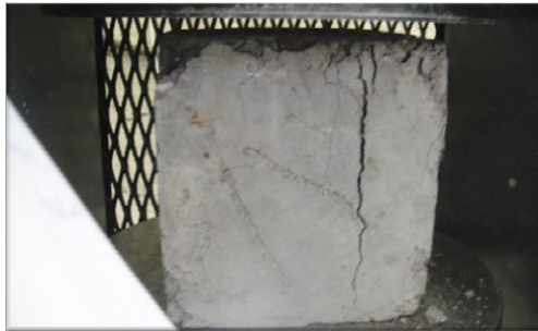
Figure 11. The shape of failure after loading for cube without GL51 and fired for 1hr
