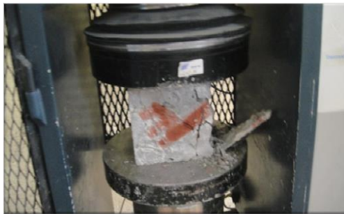
Figure 15. The shape of failure after loading for cube without GL51 and fired for 3hr
