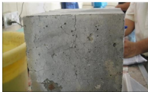
Figure 5. The surface of the cub with GL51 after 2 hr fire
