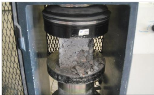
Figure 12. The shape of failure after loading for a cube with GL51 and fired for 2hr
