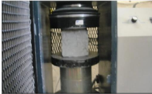
Figure 10. The shape of failure after loading for a cube with GL51 and fired for 1hr
