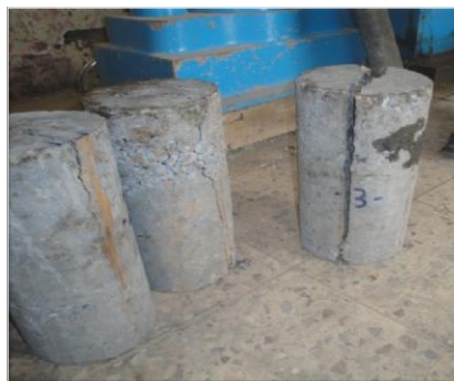
Figure 17. The shape of failure after loading for cylinder with GL51 and fired for 3hr
