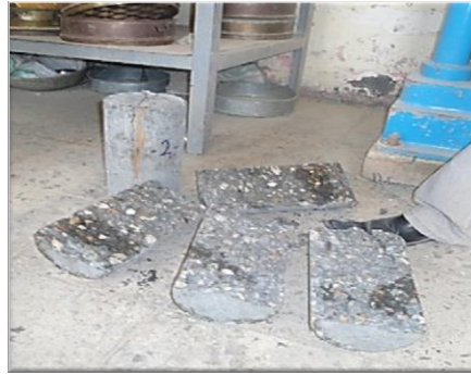
Figure 18. The shape of failure after loading for a cylinder with GL51 and fired for 3hr
