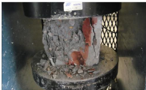
Figure 13. The shape of failure after loading for cube without GL51 and fired for 2hr
