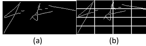
Fig. 4. Image partitioning (a) Input image (b) Image divided into 4x4 parts (zones).
