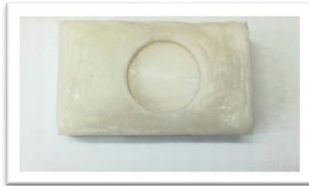
Figure (3): Silicone mold for the wax pattern fabrication.
