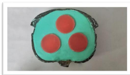
Figure (4): wax pattern for the stone mold.
