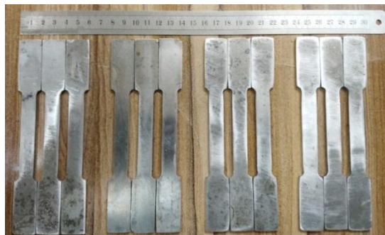
Figure-9: Tensile Test Specimens each three for specific test from right to left (Water 30min, Water 60min, Dry 30min and Dry 60min)
