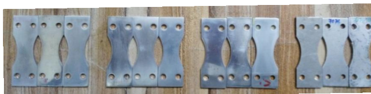
Figure-10: Fatigue Test Specimens each three for specific test from left to right (Water 30min, Water 60min, Dry 30min and Dry 60min)
