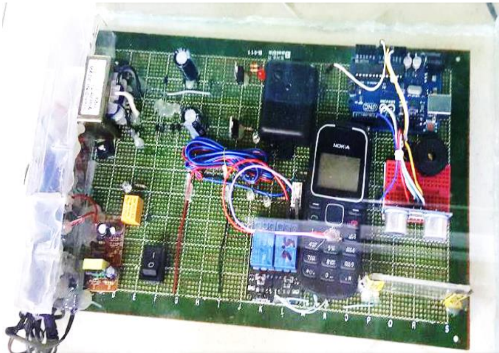
Figure (8) Snapshot of Glass Breaking Electronic Circuit Prototype.
