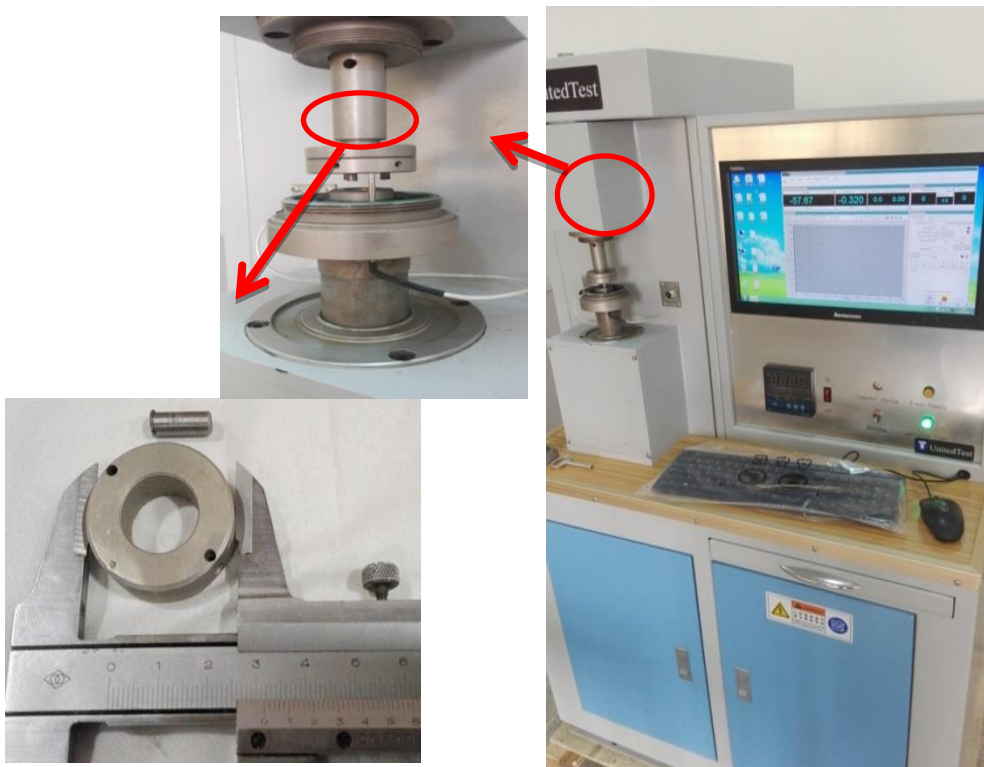
Figure 1. Vertical universal friction testing machine (MMW-1A), samples and samples fixture
