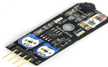
Figure (5) KY-032 Infrared Obstacle Avoidance sensor
