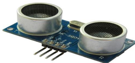
Figure (3): HC-SR04 Ultrasonic Sensor Module
