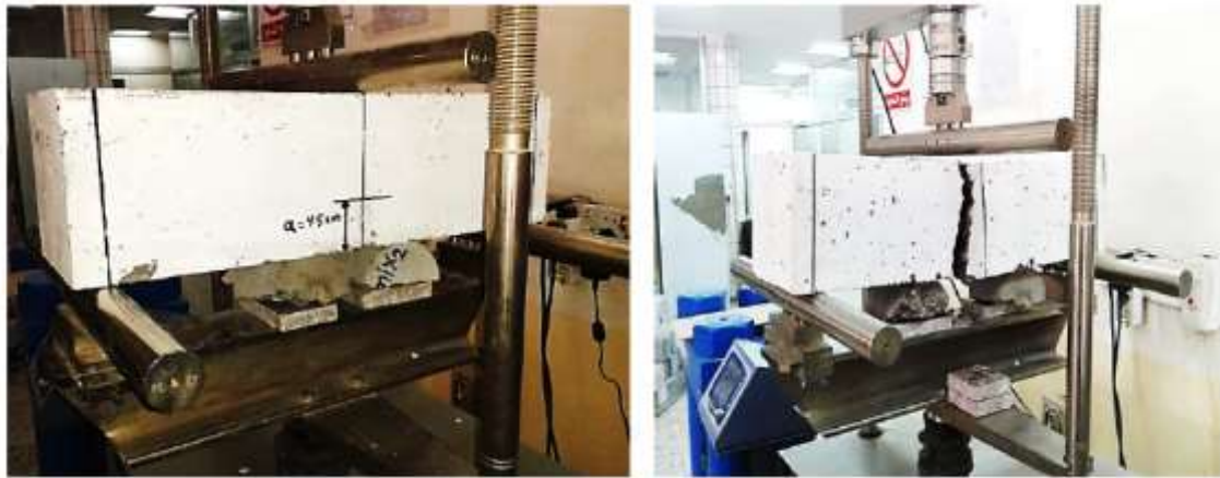
Figure (8): Beam Specimen under Test (TPBT).
