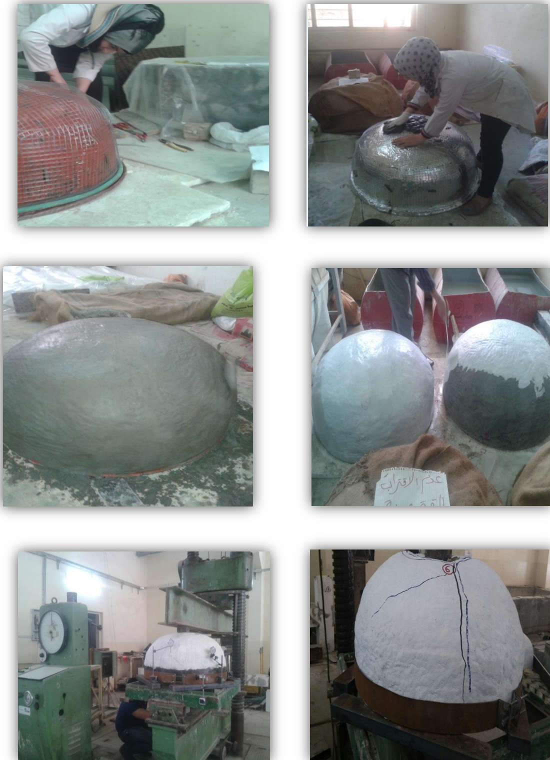
Figure. (3) Molds and Tested Domes
