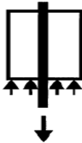
Figure (6) Pullout test [29].
