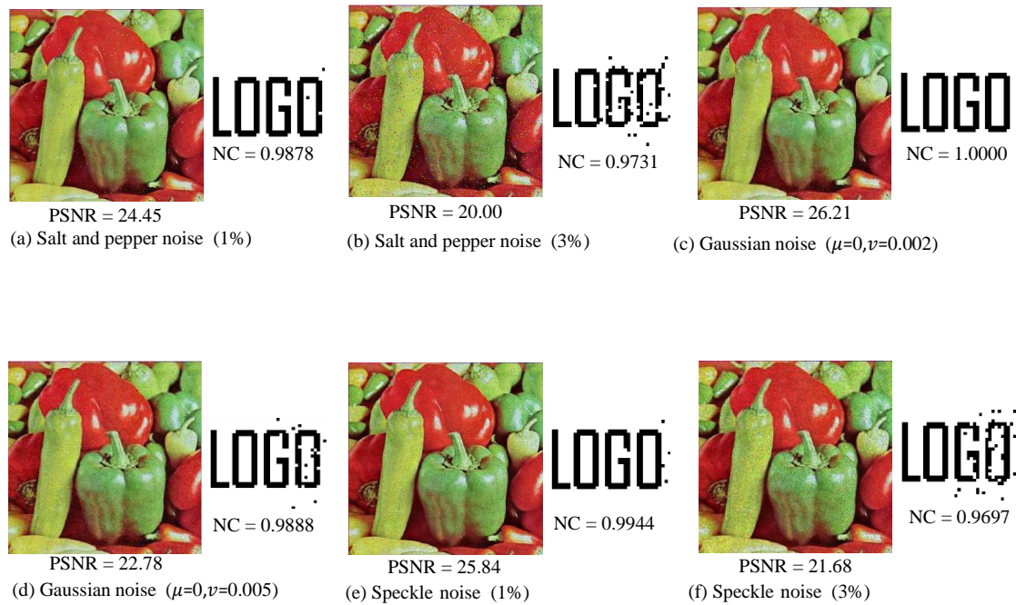
Figure 6: Watermarked Peppers images subjected to different noise attacks and the extracted watermark logo image of each one with \alpha = 0.1 .
