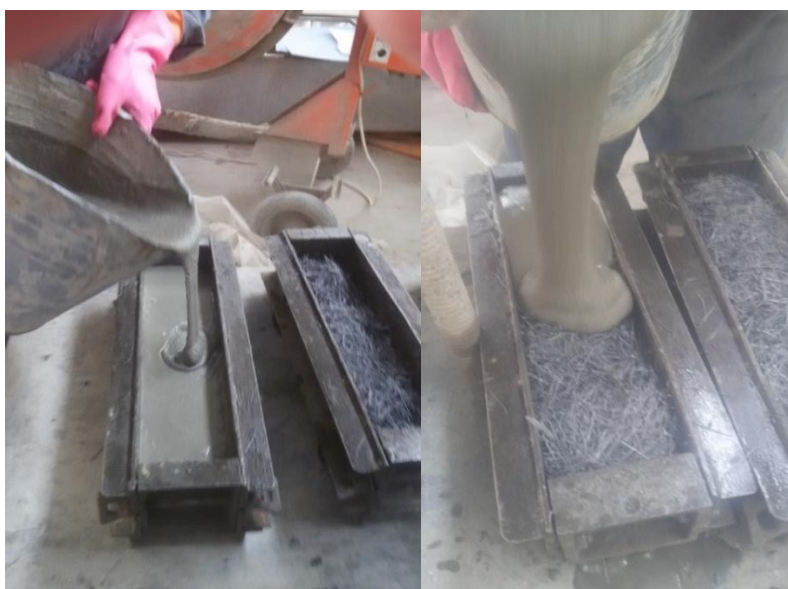
Fig (2): Casting of SIFCON mixes
