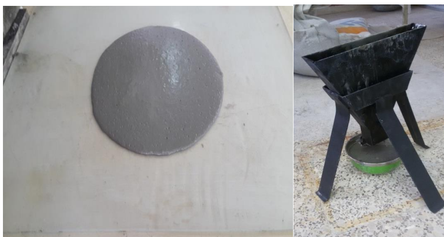
Fig (1): Mini slump flow and V-funnel tests for SIFCON mortar
