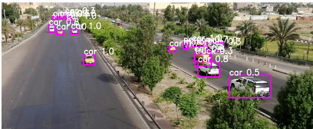
FIG. 7. VEHICLE DETECTION USING YOLO.
