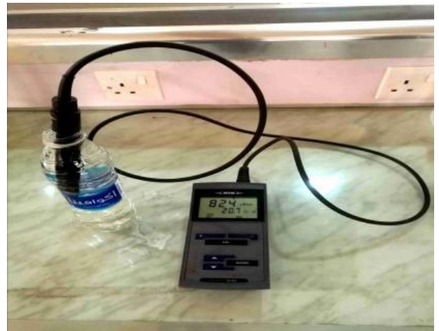
Figure 7. EC meter showing the water samples in the Abu Dali district.
