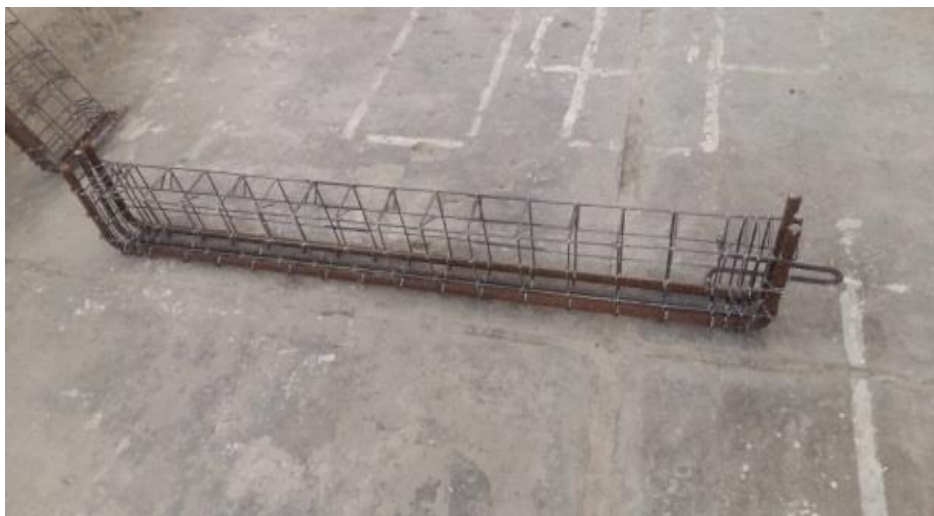
Plate 1. Steel Reinforcement Cage Used for Deep Beams.
