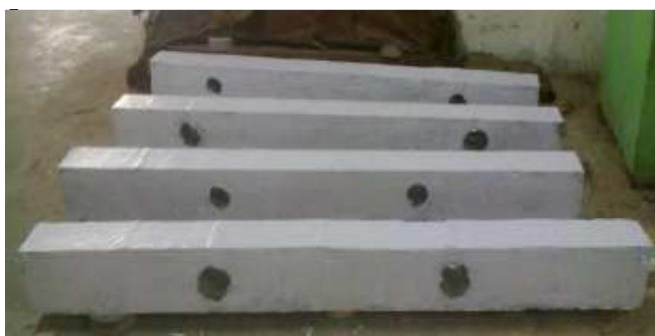
Figure 2: The beams with openings [4].
