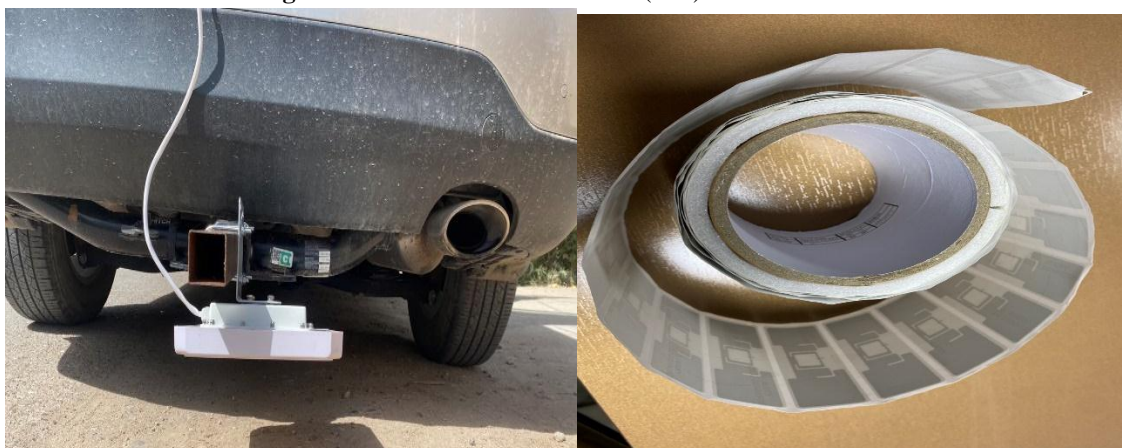
Figure 3: UHF RFID reader installed to the car and Tag
