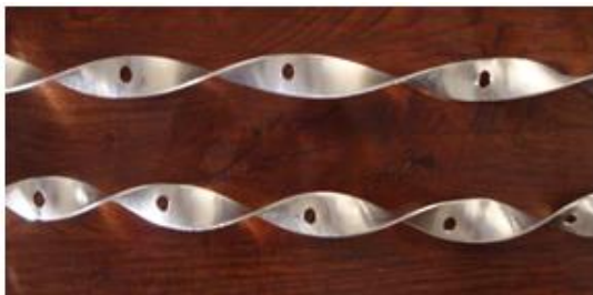
Figure 4-b. twisted tape with hole cut at different twist ratios ( \gamma=8 and \gamma=5.8 )
