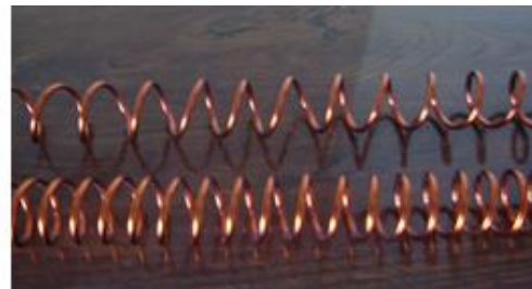
Figure 4-c. Wire coil with two pitch to diameter ratios ( CR=10 and CR=5 )
