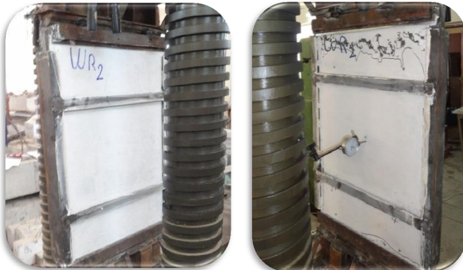
Plate (2) : RPC Wall Panels Before and After the Test.
