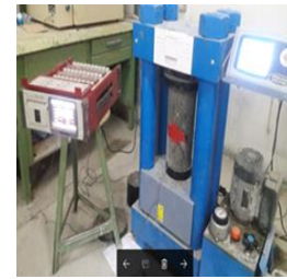
Figure.6 Test of Modules Of Elasticity
