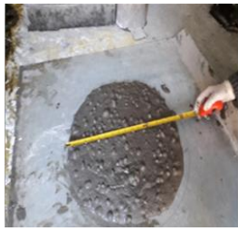
Figure.5 Test of Flow
