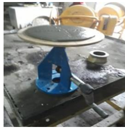
Figure.5 Test of Flow
