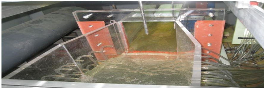
Figure 1. Channel expansion and pressure taps through the wall and connected to piezometers.
