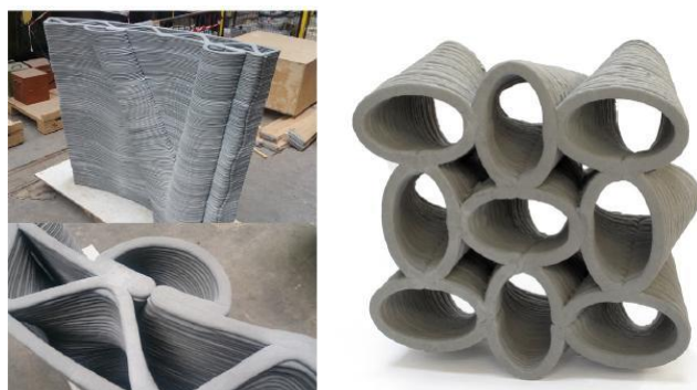
Figure 5: 3D printed large-scale structural elements with complex geometries [22]
