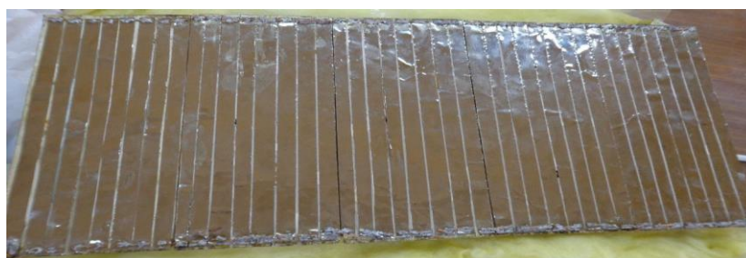
Figure (2) 40 strip heater (stainless steel foil)
