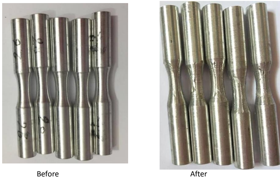
Figure 5. Fatigue specimens before and after UIP device
