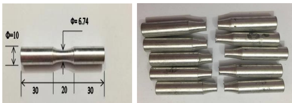
Figure 2. Dimensions of cylindrical fatigue test specimen in (mm) and Fatigue specimens after fatigue failure
