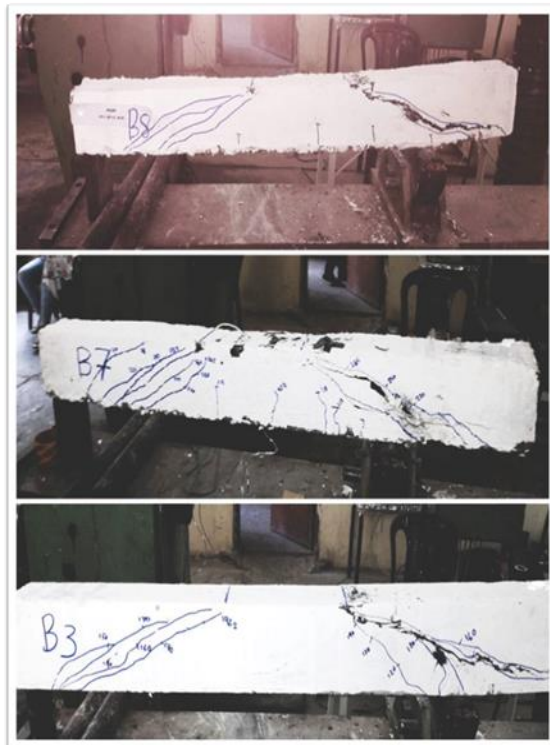
Plate (3) Crack Pattern in Group (B)
