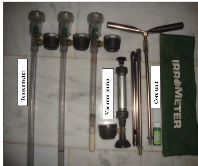
Plate (2): Three tensiometers used with its accessories
