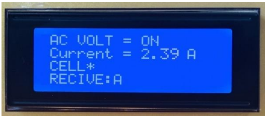
Fig. 11. Print Screen of the State of the Grid and Home for Case-A
