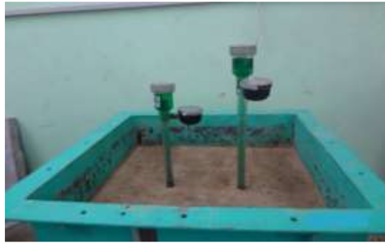
Plate 1: Measuring the matric suction of the soil by using Tensiometers.
