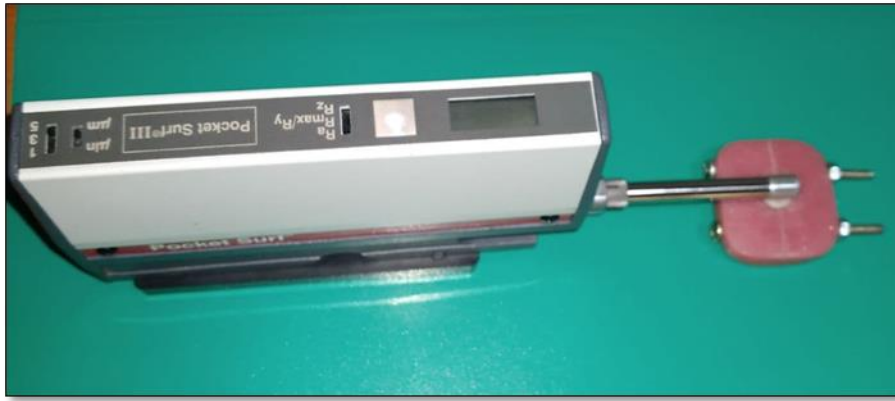
Figure (2): A contact stylus profilometer for quantitative evaluation of surface roughness with a speed of 5.08 mm/s, resolution of 0.01 \mu , stylus force of 1500 mgf /15.0 mN, and a cutoff value of (0.8 mm)
