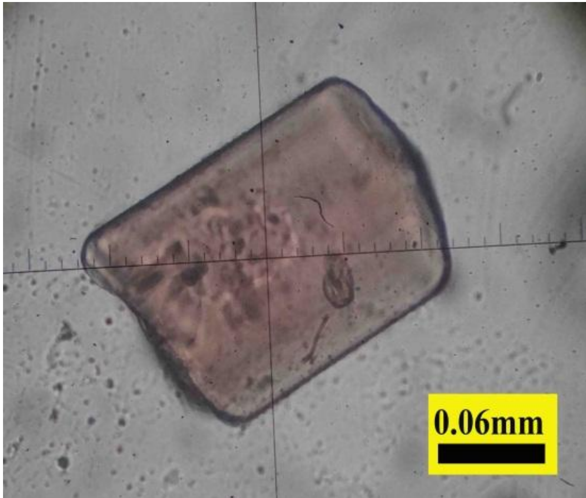
image (2) tourmaline mineral for the second horizon(Rumaiitha location) Pleochroic light brown color tourmaline, sample number R2, PPL.
