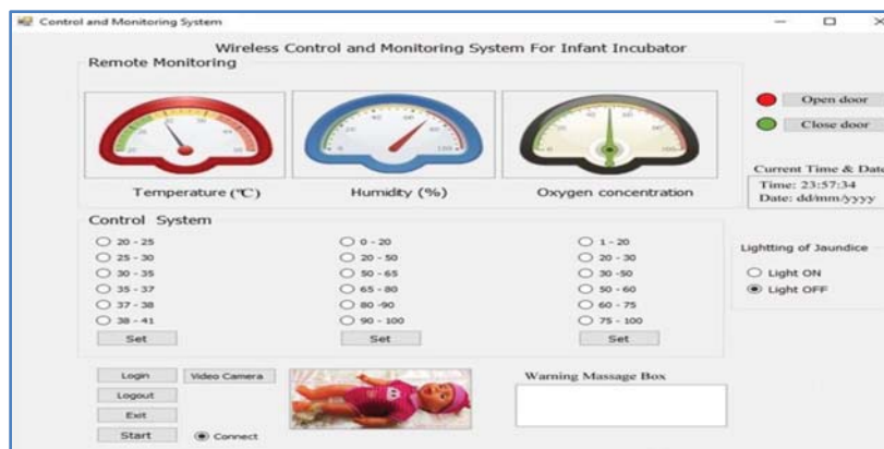
Figure 7: Main Page of Control and Monitoring System.
