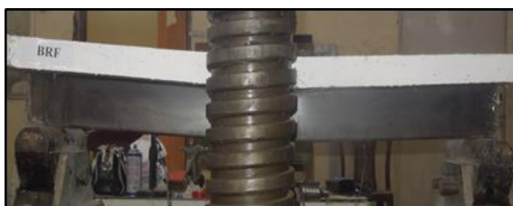
Figure 16. Mode of failure of beam BRF
