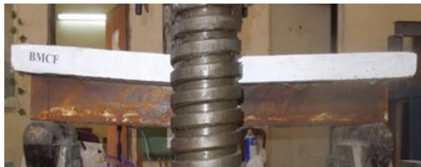
Figure 14. Mode of failure of beam BMCF
