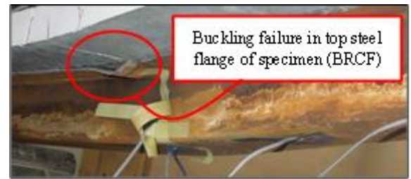
Figure 17. Mode of failure of beam BRCF
