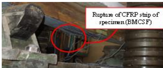
Figure 15. Mode of failure of beam BMCSF
