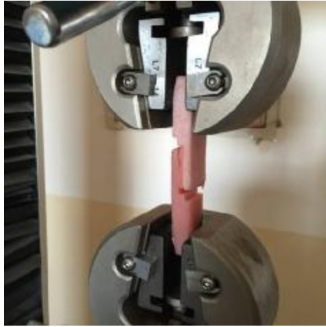
Figure 1: Testing shear bond strength specimen
