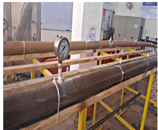
Figure 1. Main polyethylene pipe.
