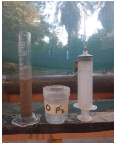
Figure 8. Withdrawal of the pollutant from the soil
