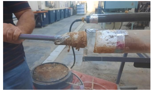
Figure 5. Filling and compacted process.
