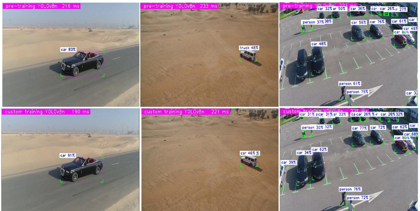
Figure 7-6: Comparing the custom-trained model with the pre-trained model
