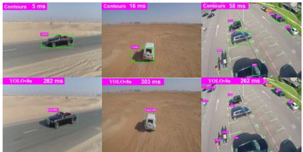
Figure 7-3: The different speed between detection and classification algorithms
