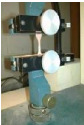
Figure 5. Specimen under tensile tester
