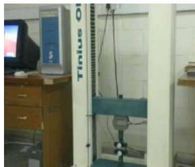
Figure 4. Tinius Olsen tensile machine
