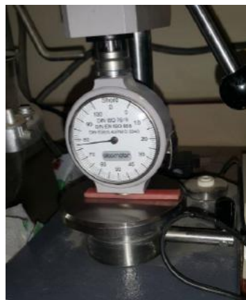
Figure 3. Specimen under hardness tester
