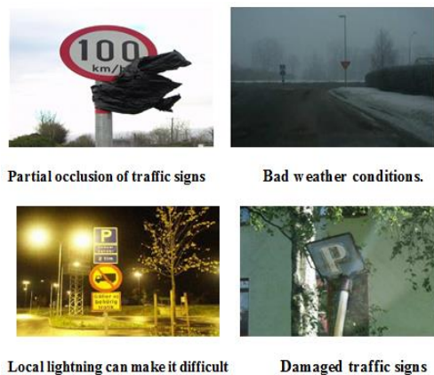
Figure (2): Potential Difficulties Traffic Signs
