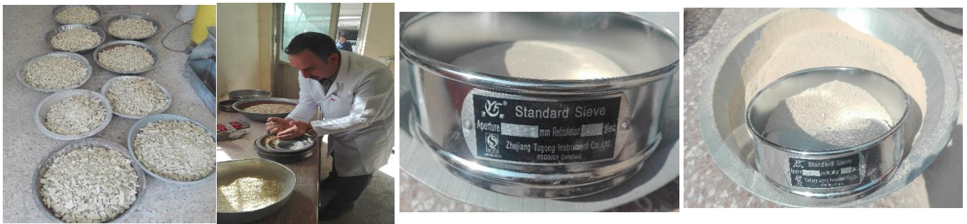
Plate 2. Step's of sieving and grains passing through 75µm
