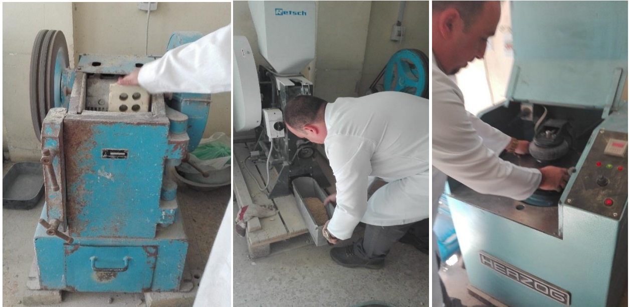
Plate 1. Step's of crushing and grounding the WCBs
