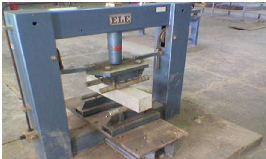
Fig .(3) Modulus of rupture Test Machine
