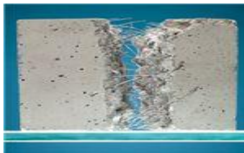
Fig . (1) Steel fiber in Concrete.
